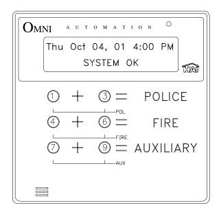
**NOTE:** The Emergency keys are always armed. The Fire and Auxiliary emergency alarms are silenced by pressing the '\*' key. To cancel a Police emergency alarm you must press the Off key and enter your code.
